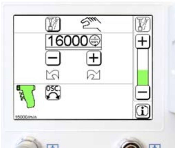
Fig. 32 The symbol "Display for oscillating or tapping mode" is illuminated in the motor control field.
